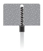
The head of the anchor should be set flush with the base material.
